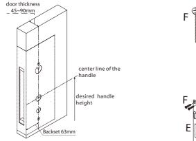
Note 1: Align the template along the vertical center line of the mortise (E) at the desired handle height, and tape it to door.
